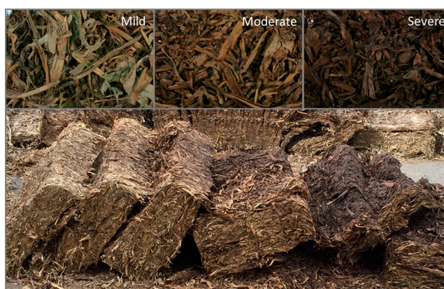
Figure 1. Dissection of bale demonstrating a range of biologically degraded regions. Grab samples were collected from mildly heated (control), moderately heated (browned), and severely heated (almost black) sections of the bale.
